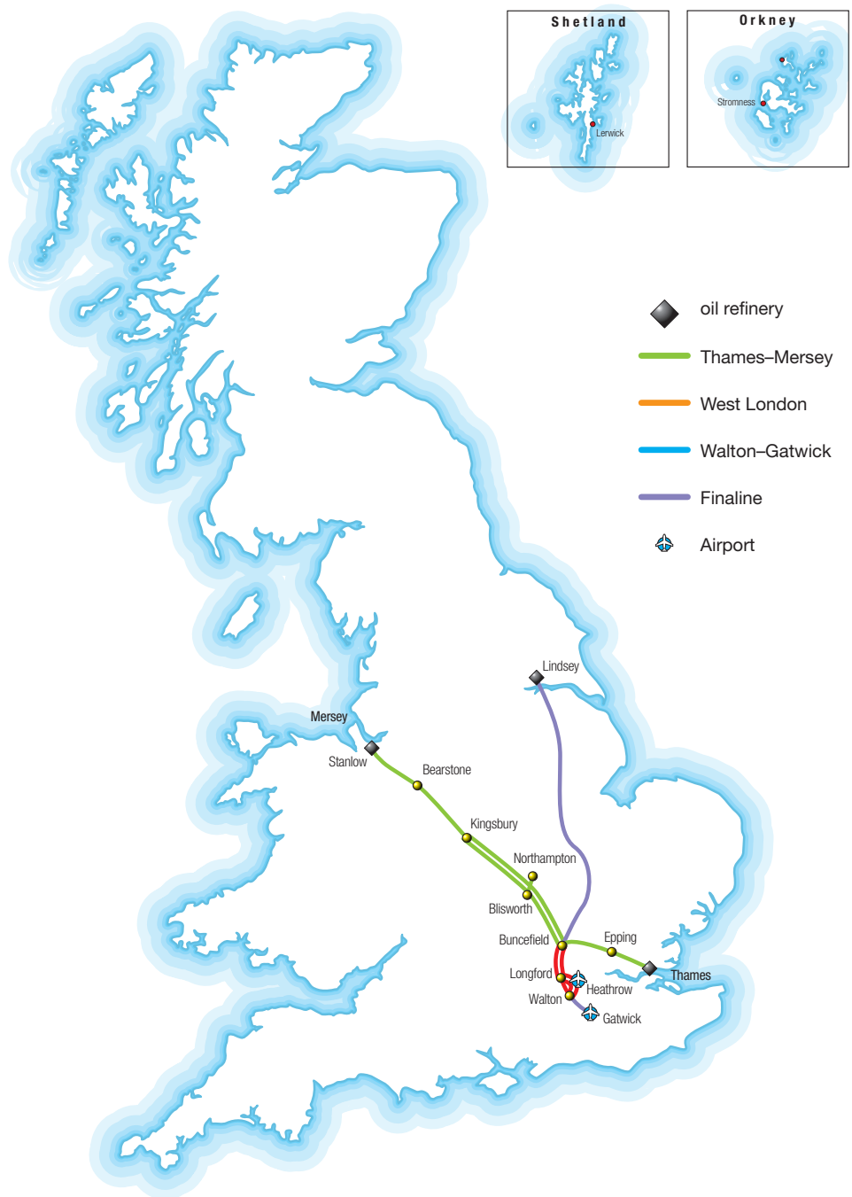
Figure 4 Schematic showing the pipeline system supplying Buncefield
